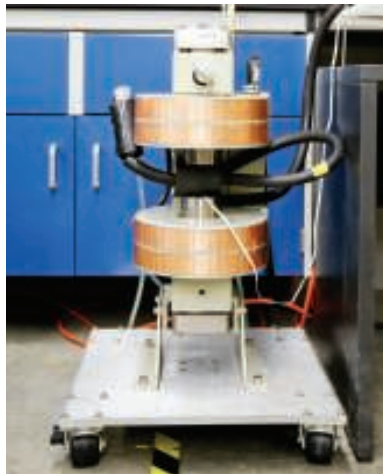
FIGURE 2. The magnetocaloric refrigeration system being developed at ORNL uses a magnetic field to remove heat
