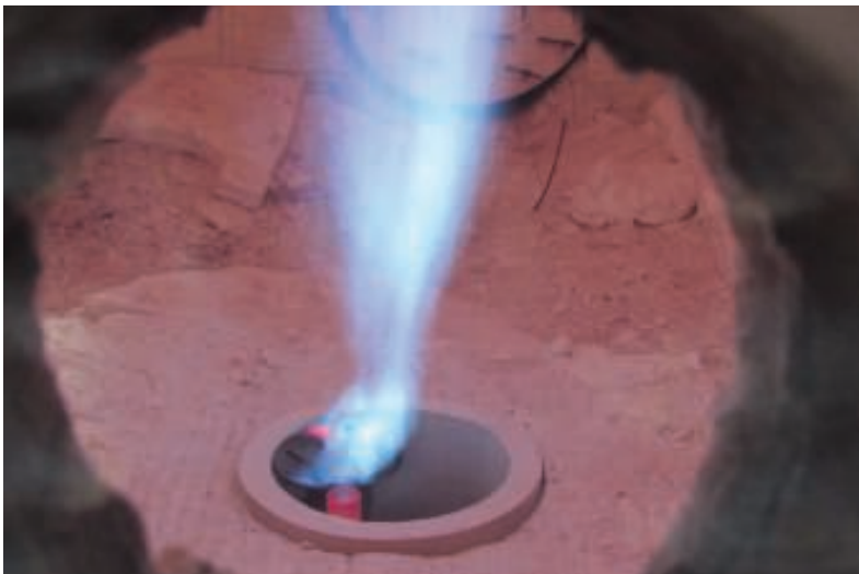
FIGURE 2. The GB Single Jet burner is a staged, round-flame low-NOx burner that uses a non-symmetrical design to boost internal fluegas recirculation and staged air and fuel to reduce NOx emissions
