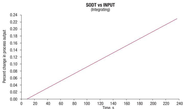
FIGURE 3. Integrating, or non-self-regulating process variables do not settle into a new steady-state value within allowable operating limits
