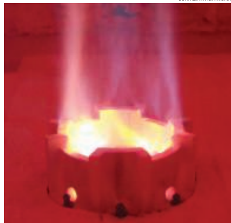
FIGURE 1. The COOLstar burner applies internal fluegas recirculation and fuel staging, which results in stable, compact flames and low NO x emissions
