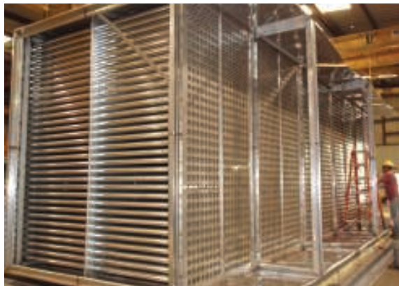
FIGURE 5. Epcon specializes in creating systems that employ heat-recovery techniques, such as this fabrication of a custom high-efficiency tube-and-shell, air-to-air heat exchanger.
